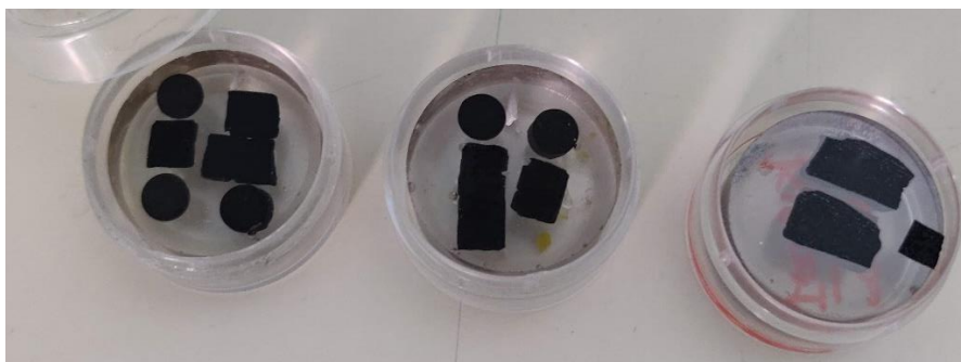
Fig. 3.6. Polished sections prepared from thermally matured KCF mudstones cylinders
