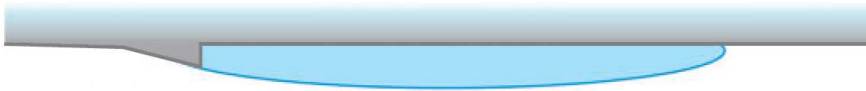
Figure 2.16 – Schematic of a partial cavity flow over a non-axisymmetric object (adapted from Ceccio 2010). The cavitator protrudes into the flow generating a cavity that downstream reattaches to the surface. The flow is from left to right.
