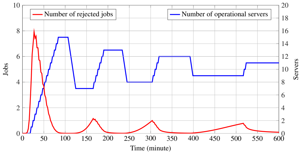
Figure 3.12: The evolution of the number of operational servers (blue) and the average of rejected jobs (red) during the first 600 minutes of the first period T_1 .
