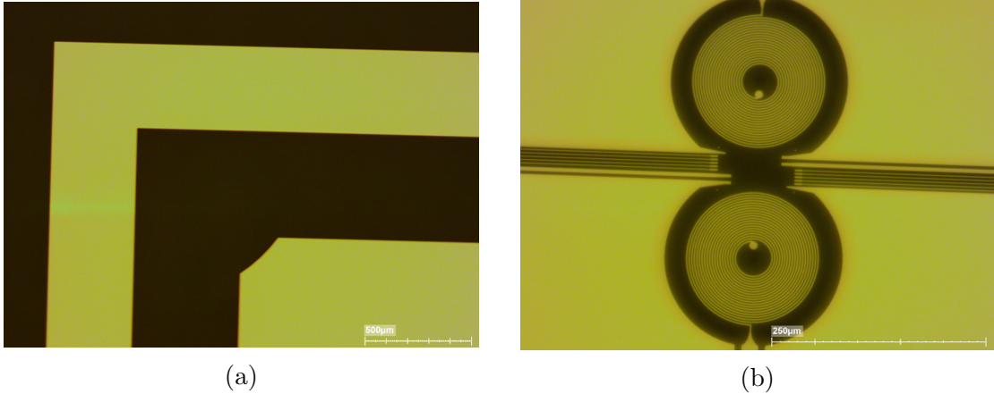
Figure A.1: Micrograph pictures of the photo masks (RFTv2) used for the optical lithography of the micron-scale planar coils (A-series). Shown are (a) the edge-bead removal (EBR) mask and (b) the mask for the coil. Yellow coloured areas correspond to the chromium/chromium oxide on the transparent quartz substrate.
