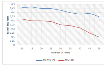
Figure 6.11 – Influence of the network size on the packet loss ratio
