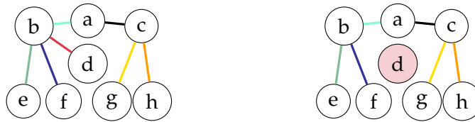
(a) IoT AJ MTD network: every pair of nodes use unique PHY parameters. (b) Insider attack: node d compromised. Jamming resilient PHY layer links.
