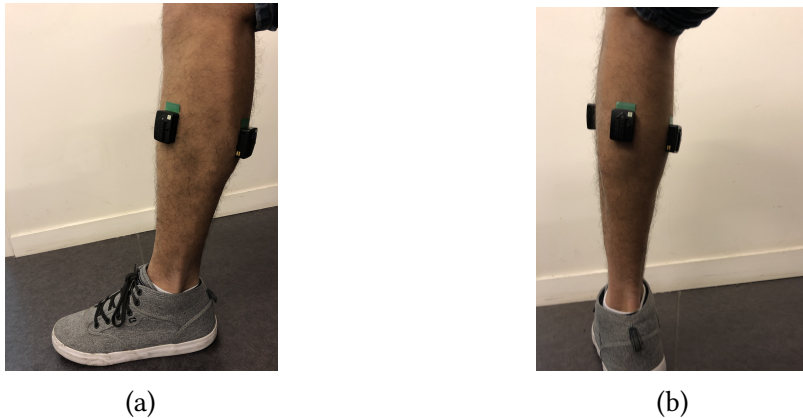
Figure 3.6 – Electromyography sensor placement to measure the tibialis anterior and gastrocnemius muscular activities.
