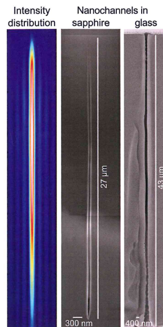
Figure 1: Bessel beam intensity distribution and corresponding nanochannels processed in sapphire and glass using single shot illumination with ultrashort lasers, observed with a Scanning Electron Microscope (SEM) apart to define a cleavage plane along a line, and we can do this with extremely high speed. This process then defines a weakened plane in the material which yields mechanical cleavage under small bending as shown in Figure 2. With industrial lasers operating at repetition rates of several hundreds of kilohertz, the nano-drilling step can reach speeds on the order of meters per second. Importantly, the width of the illuminated path, called "street" in wafer dicing technologies, is below 2 microns, saving a great deal of material waste when compared with scribing techniques.
