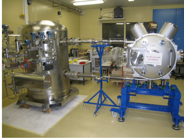
FIGURE 3.3: XEMIS2 experimental setup at the Subatech laboratory: on the left the cryostat and on the right the camera.
