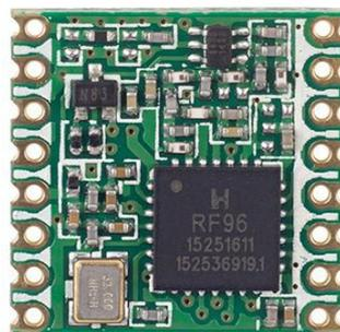
**Figure 3.10** *Module LoRa RF96*
