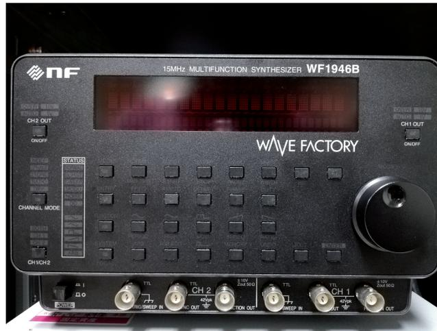
Figure 3.9: Front view of the WF-1946B multifunction synthesizer.
