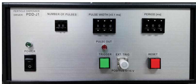
Figure 3.6: Front view of the pulse generator which is used to control the injection of the dust particles.
