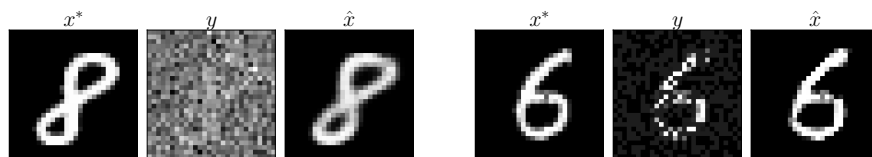
Figure 3: A ground truth image \mathbf{x}^* is corrupted and results in an observation \mathbf{y} for (Left) a denoising task and (Right) an inpainting task, from (Baker et al., 2020). The goal is to reconstruct the ground truth signal \mathbf{x}^* from the observation of \mathbf{y} . As an illustration, \hat{\mathbf{x}} may be the output of a machine learning reconstruction.
