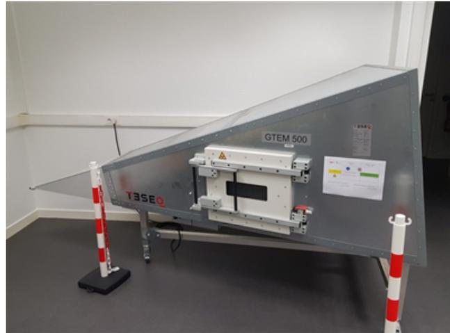
Figure I.37 – Cellule GTEM [72].
