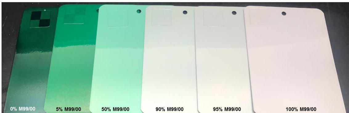
Figure 5-6: Panels from Range 2 with different percentages of aluminum tinting base, M99/00, in green tinting base
