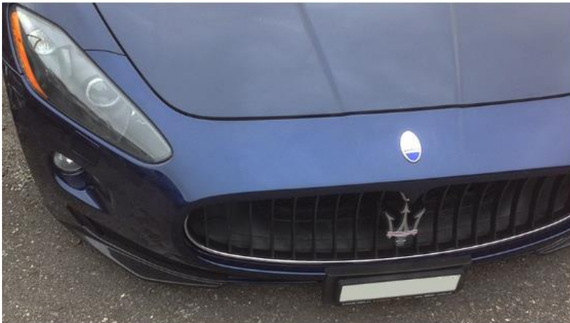
Figure 1-2: Noticeable color differences between the aisle, the hood and the bumper after repair (Carrosserie-Geneve.Ch, 2015)
