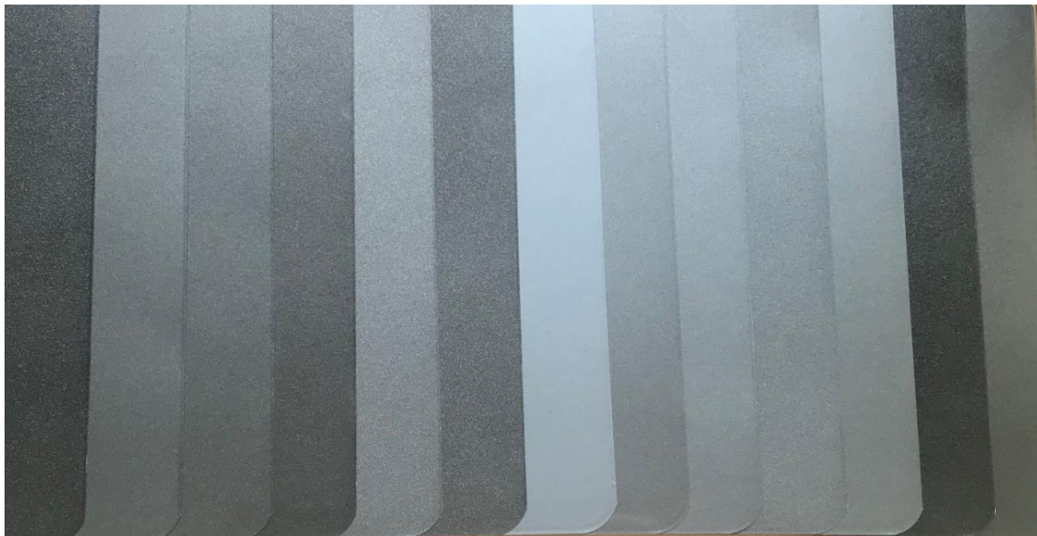
Figure 5-18: Image of the thirteen panels from Range A, 60% Alu + 40% A926
