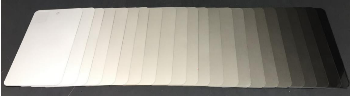
Figure 5-2: Letdowns of M99/00 with A926, from 100% to 0% of aluminum tinting base content
