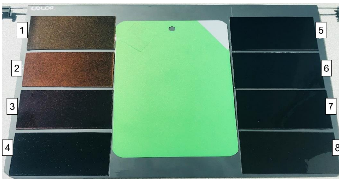
Figure 5-31: Panel holder used for Color evaluation with the eight standards (where #1 = C_1 - Color_Gold, #2 = C_2 - Color_Orange, #3 = C_3 - Color_Red, #4 = C_4 - Color_White, #5 = C_5 - Color_Green, #6 = C_6 - Color_Blue, #7 = C_7 - Color_Violet and #8 = C_8 - Color_Aluminum)
