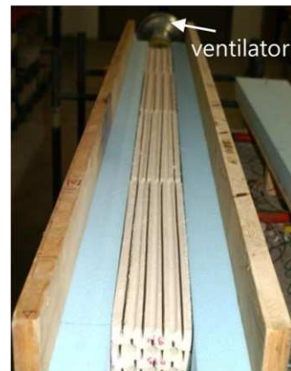
(b) concrete blocks of 16 slabs of 50 \times 10 \times 3 \text{ cm}^3 by sorption of humid air (90 % RH)
