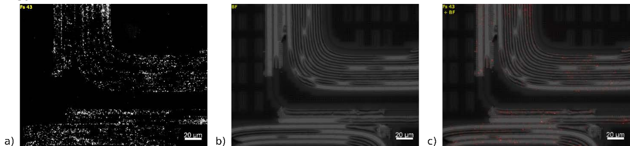
Figure 6.22 result of the differential functionalization. a) image of the fluorescent light, b) image of the visible light where the lighter part is the Au, superposition of the two where the red points are the fluorescent light of the nanoparticles.
