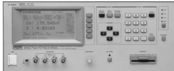
FIGURE II.36 – HP 4284A Precision LCR meter
