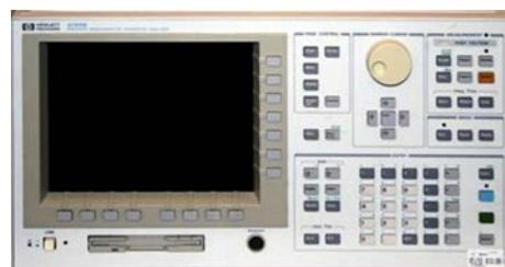
FIGURE II.40 – Agilent 4156B Semiconductor parameter analyzer.
