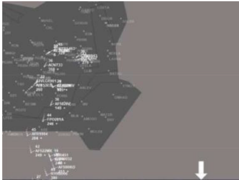
FIGURE 3.9: SmartPan: the arrow indicates a calling aircraft outside of the radar image.
