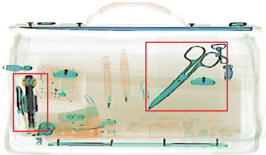
FIGURE 3.18: The real threat is the revolver on the left of the luggage
