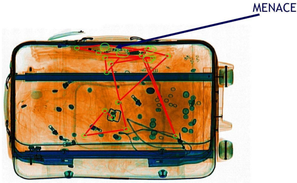
FIGURE 3.14: Interpretation errors. The security agent notice the menace at the top of the image do not interpret it as a threat (the initiating system of an explosive)
