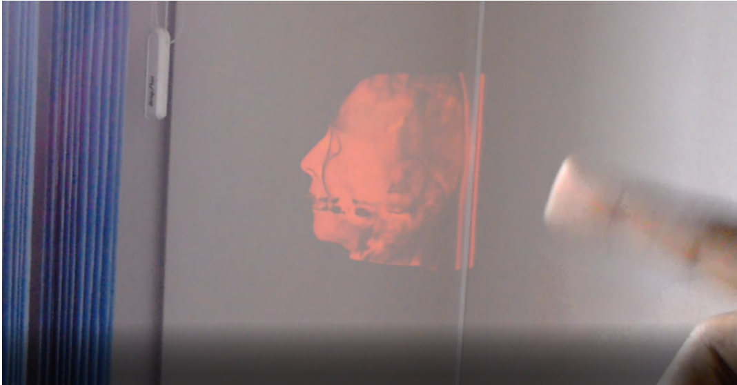
FIGURE 5.8: A head CT scan rendered on the hololens using a ray-casting algorithm
