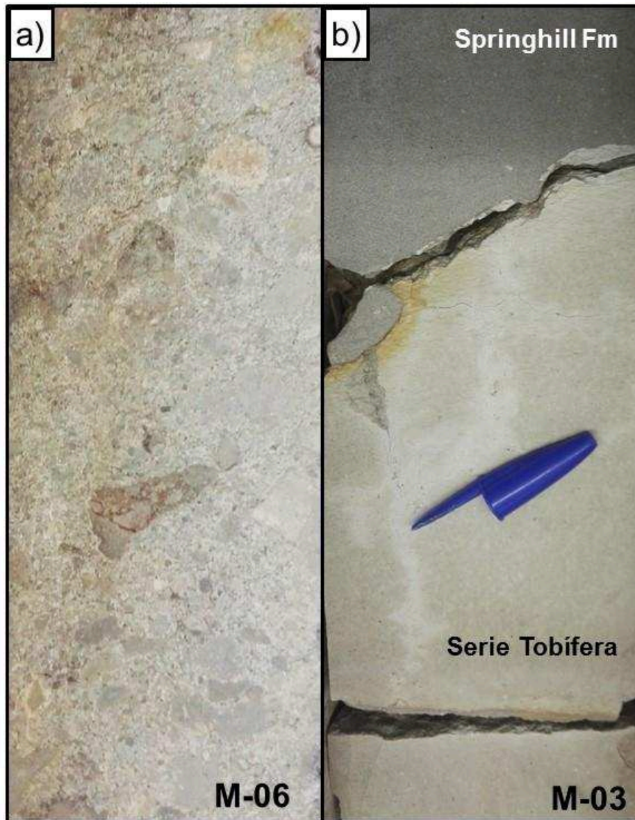
Figure 5.4: Core photos of the samples analyzed in the study: a) Sample M-06: a volcanic breccia sampled from the Erizo.x-1 well; b) Basal contact of the Springhill Fm (post-rift) overlying the Serie Tobífera, from which Sample M-03 was recovered.
