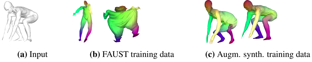
Figure 4.9 Importance of the training data. For a given target shape (a) reconstructed shapes when the network is trained on FAUST training set (b) and on our augmented synthetic training set (c), before (left) and after (right) the optimization step.
