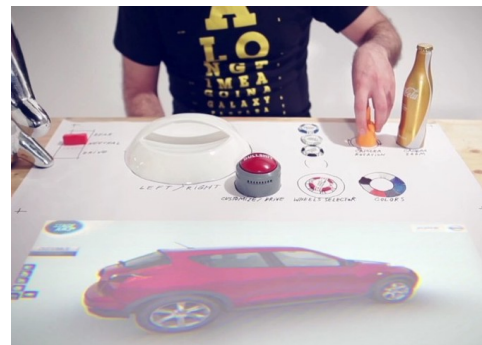
(f) Smart humans controls: Using action detection, Ayotle turn physical objects into a tactile interfaces. a
