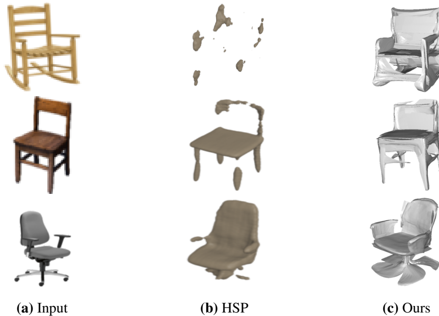
Figure 3.6 Single-view reconstruction comparison on natural images. From a 2D RGB image taken from internet (a), HSP Häne et al. (2017) reconstructs a octree-based 3D model (b), and our AtlasNet a triangular mesh (c).
