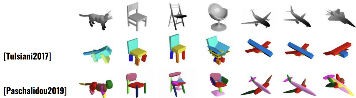
Figure 2.12 Primitive-based reconstructions. Figure from Tulsiani et al. (2016) and Paschalidou et al. (2019) . Primitive reconstructions are structure, parsimonious and provide part correspondence across shapes.
