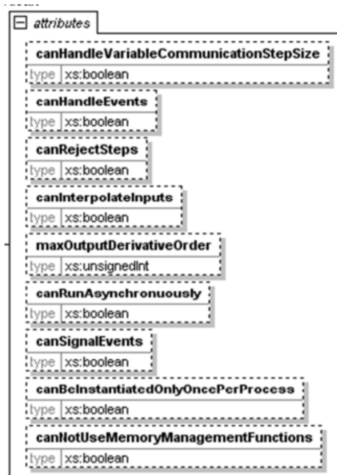
Figure 17: Capability flags of FMI for Co-Simulation
