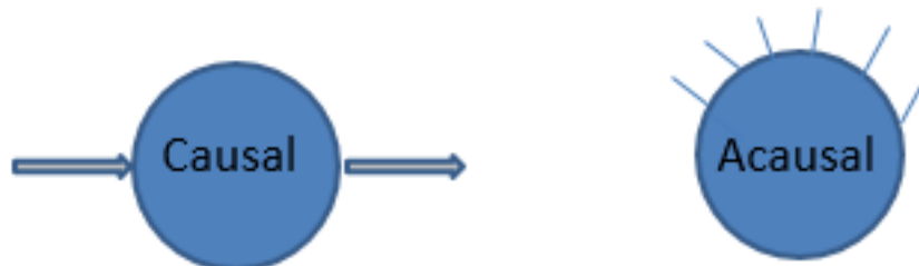
Figure 8: causal approach (oriented) / acausal approach (unoriented)
