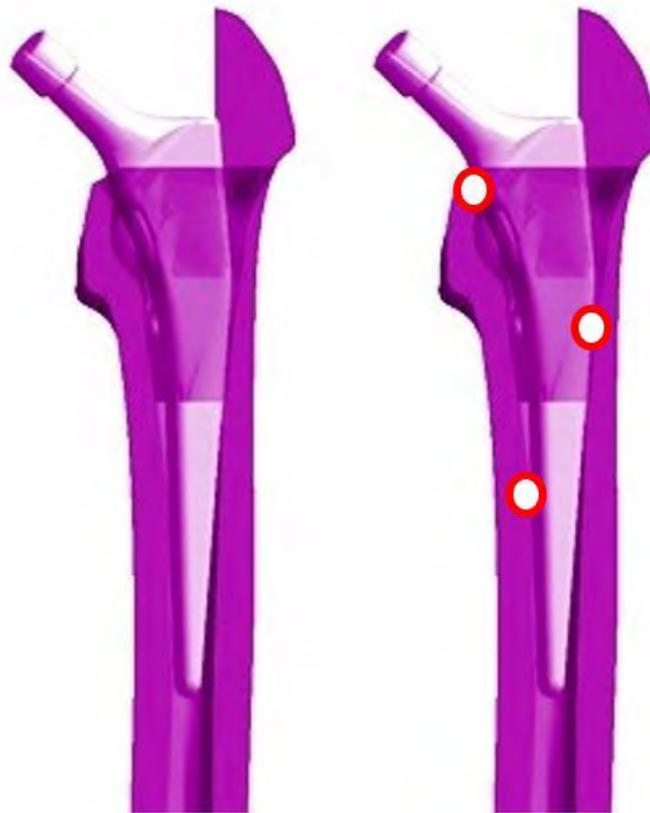
Figure 2.5. Contact between the right hip stem and the femoral canal
