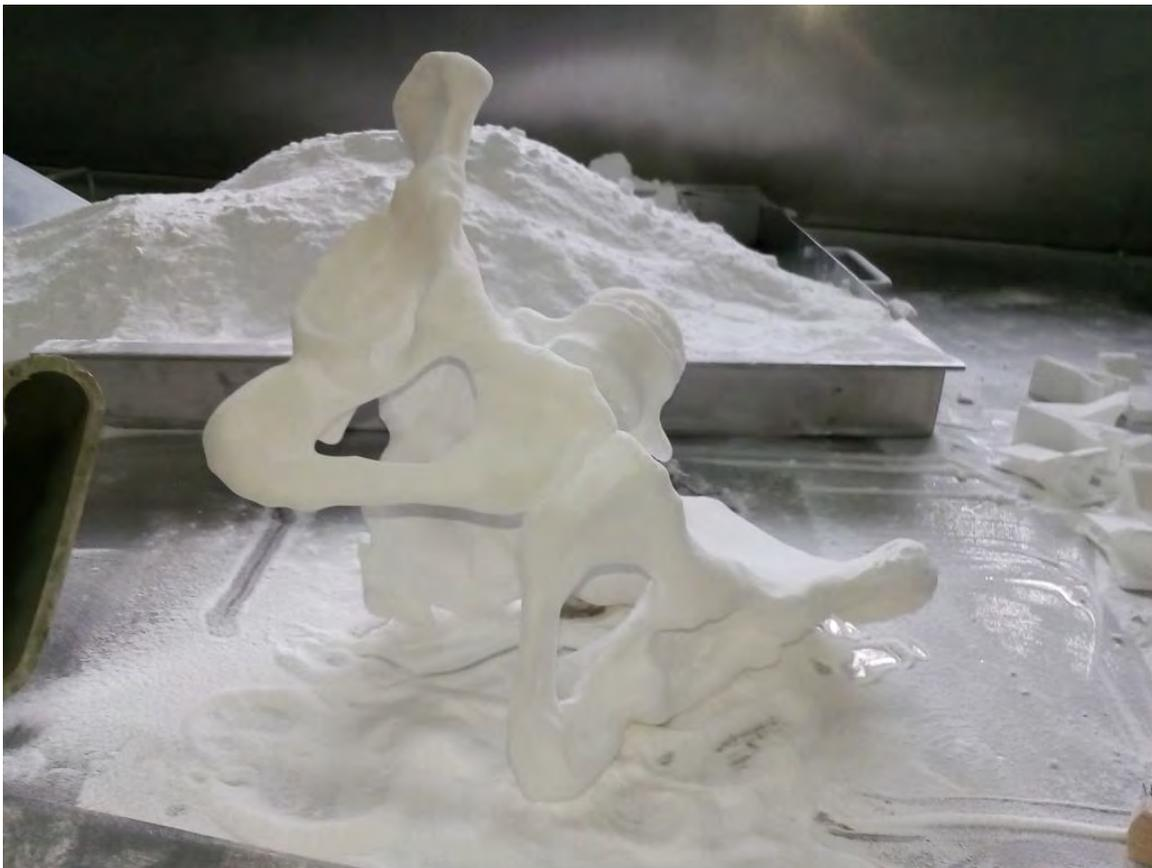
*Figure 1.4. Pelvis model manufactured with AM technology*
