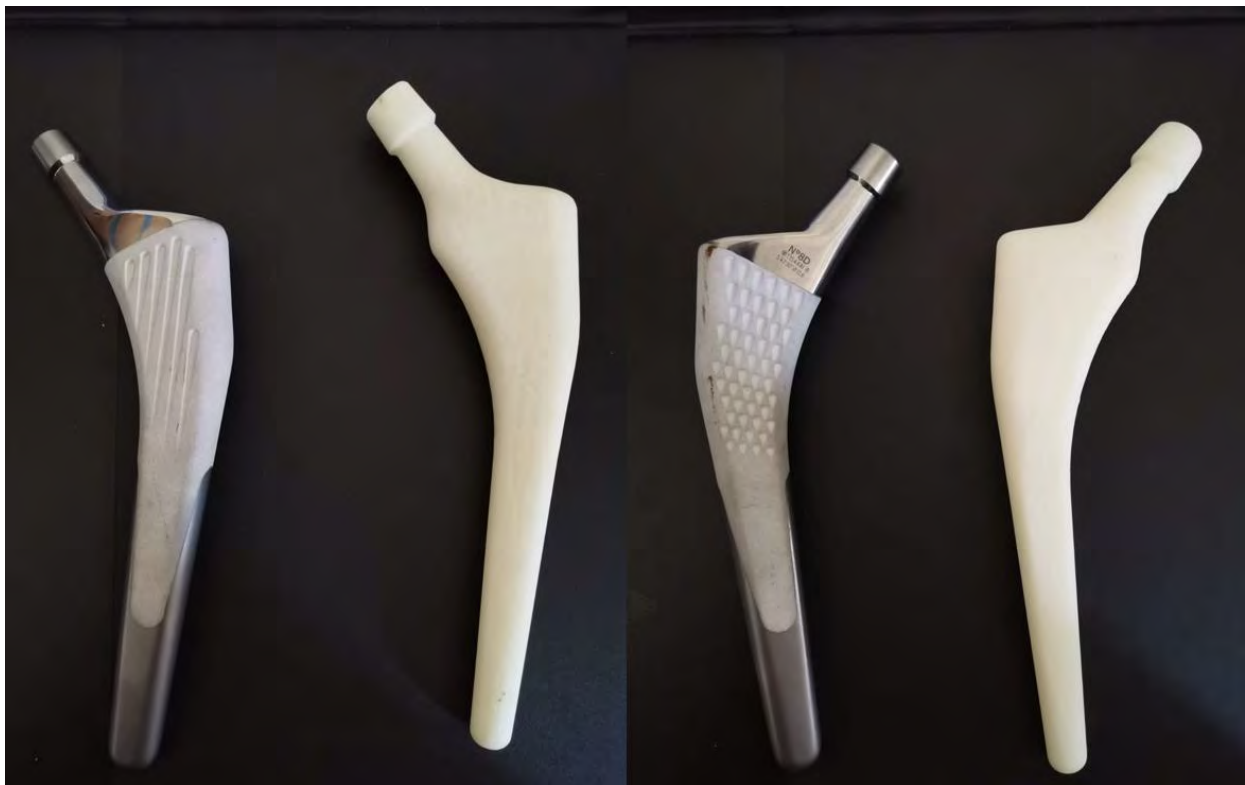
Figure 6.4. Comparison of the manufactured prototype and a commercial hip stem (Linea Anatomical hip system Tornier©)
