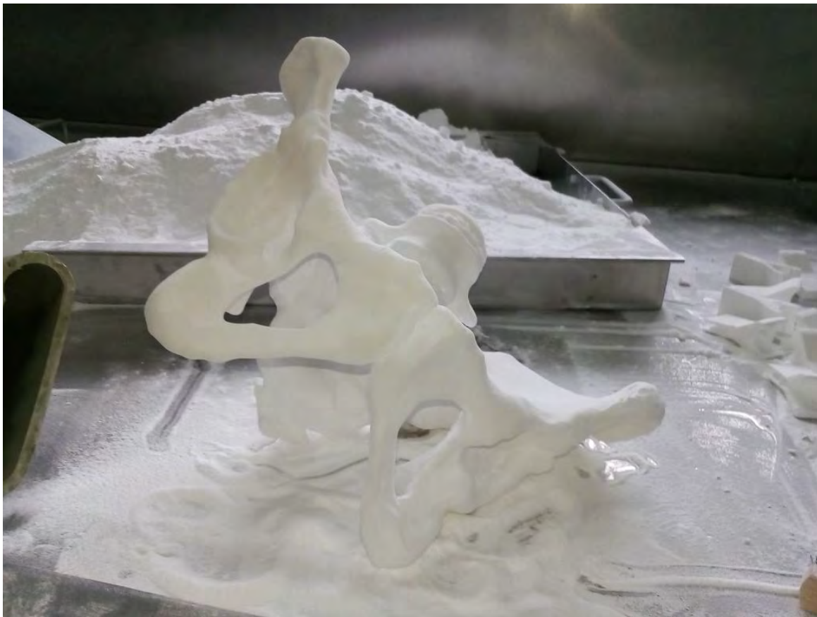
Figure 1.4. Pelvis model manufactured with AM technology
