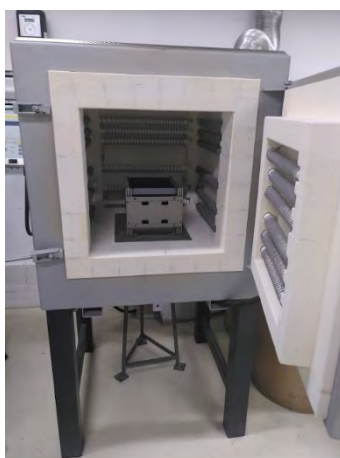
Figure 3.37. Nabertherm chamber furnace with the wafer carrier positioned inside
