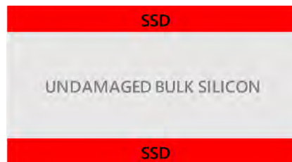
Figure 1.16. Schematic cross section view of an as-cut DWS silicon wafer
