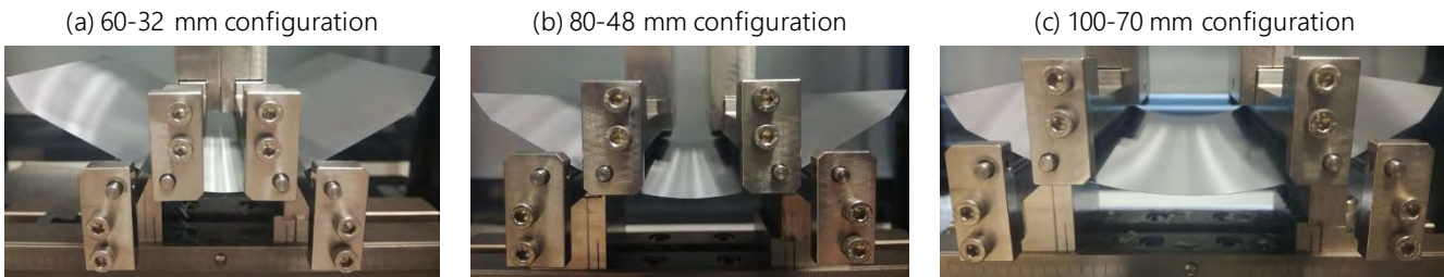
Figure A.2. The three configurations used for the 4-line bending tests
