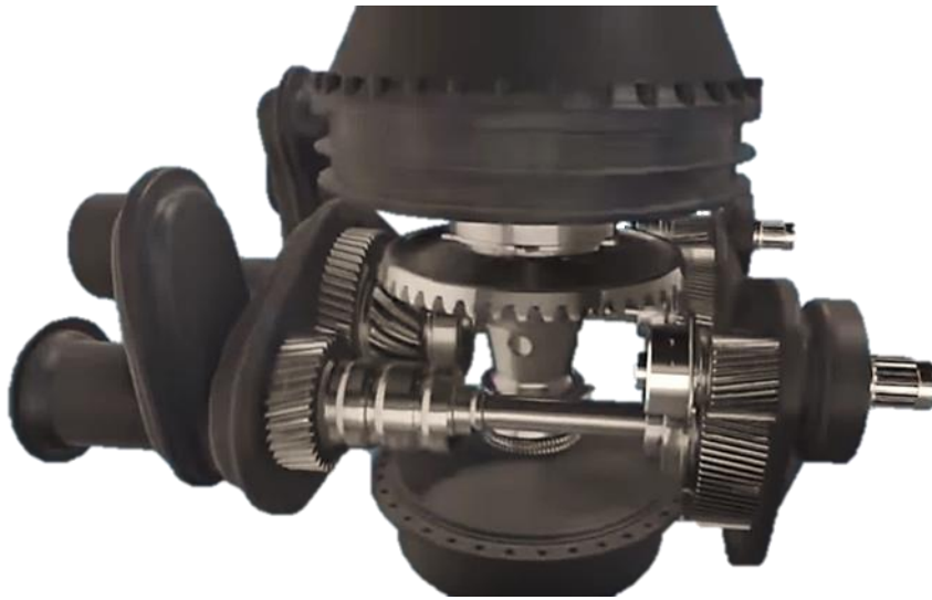
Figure I.1 : Scheme of a Helicopter main gear box and its components [21]
