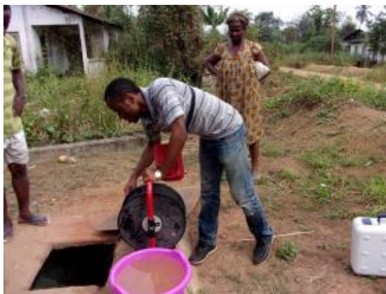
Figure 13: measurement of water table in a hand-dug well.
