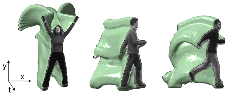
Figure 1.4 – Space-Time Shapes (STS) of “jumping-jack”, “walking” and “running” actions (Gorelick et al., 2007).
