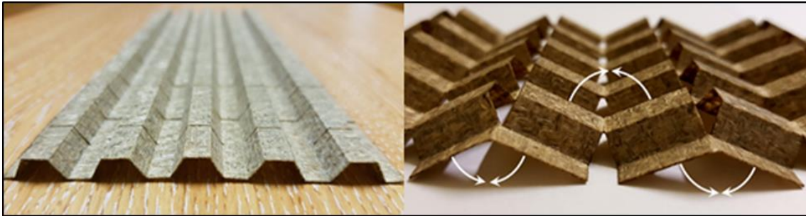
Figure 7 - Natural fibre kirigami corrugated sheet and its folding process[23]
