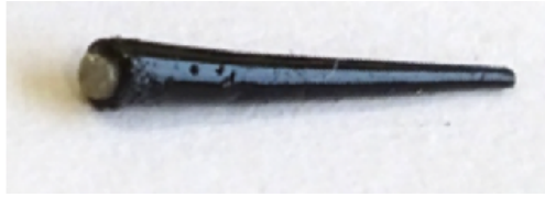
Figure 4.1: Flexible magnetic swimmer used in the experiments
