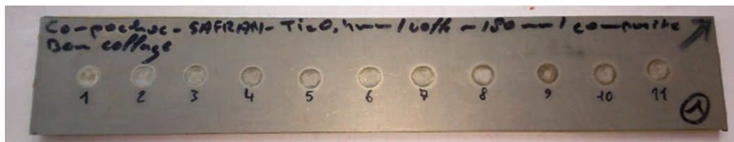
FIGURE 64 – Assemblage TA6V4/Epoxy/Composite tissé 3D - Dimensions latérales 240 mm x 40 mm.
