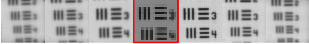
(b) Stingray 1.0: gr3 - el3 , from z = 227mm to z = 239mm , steps of 2mm .
