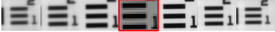
(b) Stingray 1.0: gr2 - el1 , from z = 227mm to z = 239mm , steps of 2mm.
