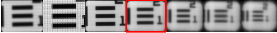
(c) Stingray 2.0, a>0 : gr2 - el1 , from z = 227mm to z = 239mm , steps of 2mm.
