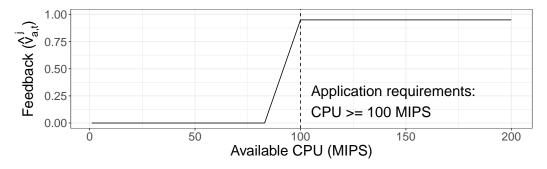
**Figure 13.11:** Estimation function ( $f_{est}$ ). Shape of  $f_{est}$  for an application that requests a CPU with at least 100 MIPS.
