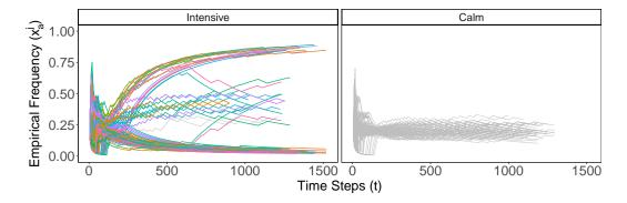
**Figure 14.6:** UCB-MC learning rate for a long duration (5h) experiment in an ill-informed environment. Each line represents the frequency an application has selected determined host  $(x_a^j = n_a^j/t)$ . We highlight with a different color, the applications that were able to identify the best hosts to run (i.e., applications whose 2 best hosts have at least 75% probability of being chosen).
