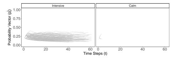
**Figure 13.10:** EXP3-MC learning rate for an experiment in a well-informed environment. The figure shows the probability vector  $p_t^j$ , each line represents the probability that an application has to select each host. Calm applications rarely exceed the threshold and so do not migrate. Consequently, the  $p_t^j$  does not evolve over time.
