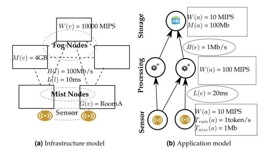
**Figure 9.3:** Components of the provisioning problem
