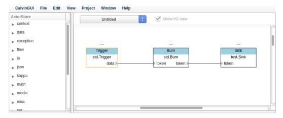
**Figure 6.4:** Snapshot of Calvin's graphical user interface used to implement an application example.
