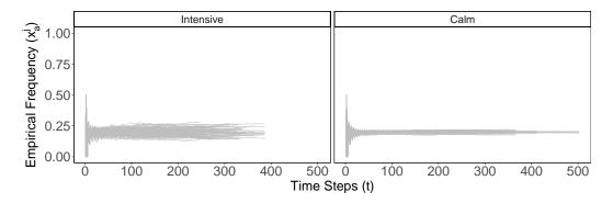
**Figure 13.5:** UCB learning rate for an experiment in a well-informed environment. Each line represents the frequency an application has selected determined host  $(x_a^j(t) = n_a^j/t)$ . We highlight with a different color, the applications that were able to identify the best hosts to run (none in this case).
