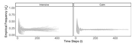
**Figure 13.8:** UCB-MC learning rate for an experiment in a well-informed environment. Each line represents the frequency an application has selected determined host  $(x_a^j(t) = n_a^j/t)$ . We highlight with a different color, the applications that were able to identify the best hosts to run (none in this case).
