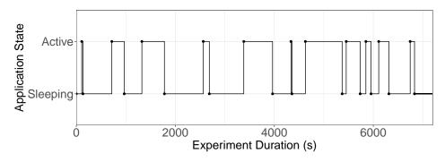
**Figure 13.3:** Workload - Churn. Example of state transitions for an application with mean active/sleeping time  $(1/\lambda)$  of 300s.
