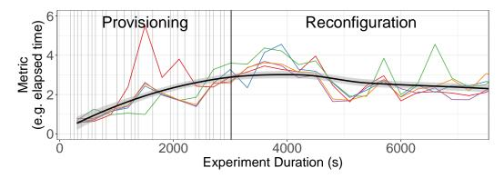
**Figure 4.4:** Studying the orchestration phases. Each colored line represents the metric for one test run. The black line represents the average performance of all runs. During the provisioning phase, each vertical gray line represents the deployment of an application.
