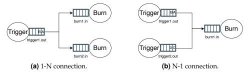
**Figure 8.3:** Internal representation of ports in actors. Each port has a queue of limited size associated. Extra configurations are available to dictate how messages are sent between source and target actors.
