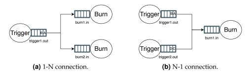
**Figure 8.3:** Internal representation of ports in actors. Each port has a queue of limited size associated. Extra configurations are available to dictate how messages are sent between source and target actors.
