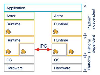
Figure 6.2: Calvin's architecture [[PA15], Figure 1 (right part)].
