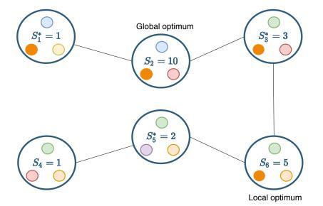
**Figure 9.2:** Set of solution generated by GRASP for a hypothetical maximization problem (higher values are better).  $S_1^*$ ,  $S_3^*$  and  $S_5^*$  are initial solutions generated by ConstructGreedyRandomizedSolution.
