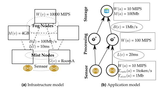
Figure 9.3: Components of the provisioning problem
