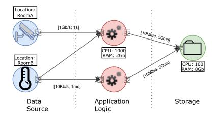
**Figure 4.3:** Graph model for a Fog-IoT application. This model represents a typical application studied in this work.
