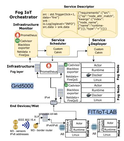
**Figure 7.1:** FITOR platform. This figure depicts the components used to build the architecture proposed in Fig. 5.1.
