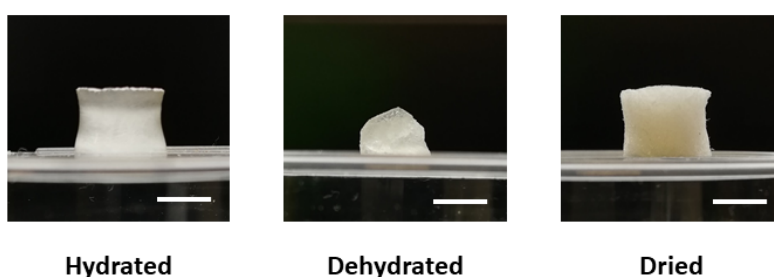
FIGURE 4.5: Photographs of cylindrical alginate cryogels in hydrated, dehydrated and dried states. Scale bar = 5 mm.
