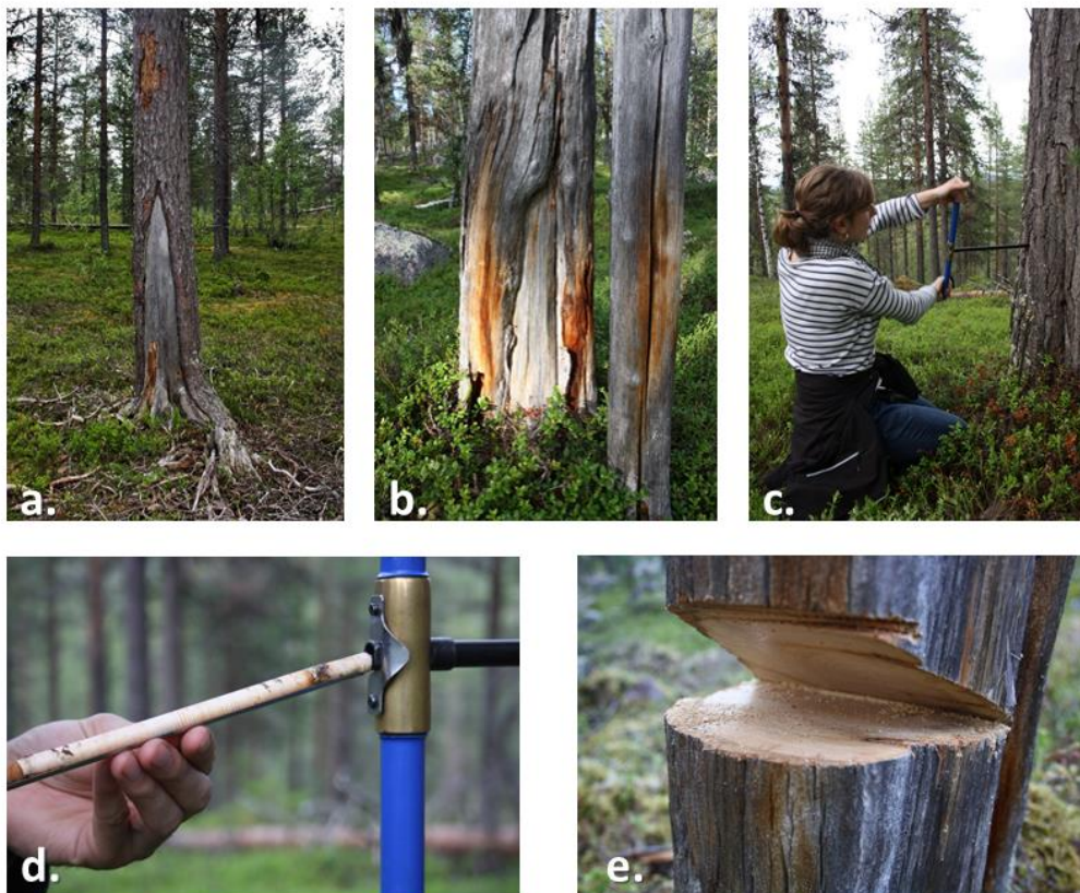
Figure 12. a. A fire scar on a living Scots pine tree; b. a fire scar on a dead Scots pine tree; c. coring into a Scots pine tree with a fire scar; d. extracting the core from the increment borer; e. after sawing a cross-section in a dead Scots pine tree with a fire scar. Photos: a, b, d, e: S. Cogos; c: S. Roturier
