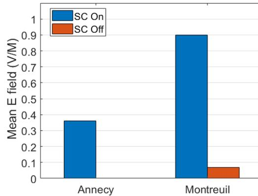
**Figure 32, Anney and Montreuil stationary mean E-field comparison. E-field values are the quadratic sum of the measured fields at 800 MHz, 1800 MHz and 2600 MHz LTE bands.**
