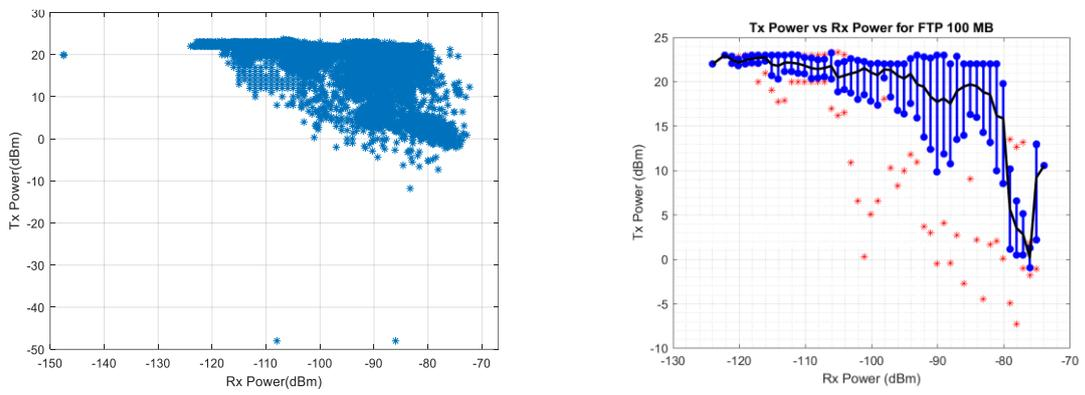
**Figure 49, LTE TX power vs RX power for VoLTE, VoIP (skype), 10 MB file transfer, and 100 MB file transfer in Basel campaign. On left figures, blue dots represent measurement points. On right figures, red dots represent the minimum and maximum measured values, blue lines represent the standard deviation and black line represents the mean value.**
