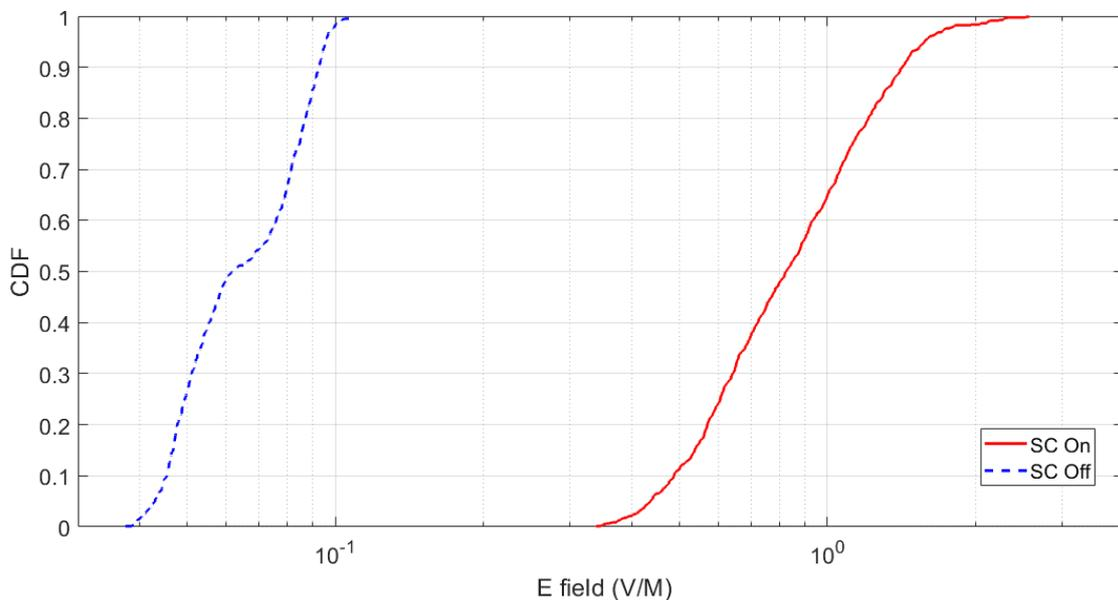
**Figure 31, CDF, Montreuil stationary E-field results for SC On and SC Off scenarios at the same locations. E-field values are the quadratic sum of the measured fields at 800 MHz, 1800 MHz, and 2600 MHz LTE bands.**
