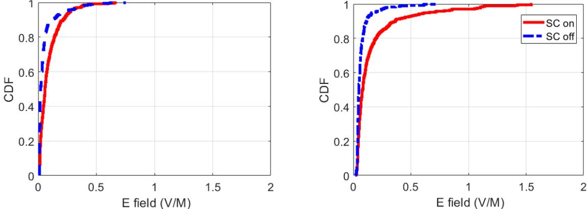
**Figure 33, CDF, Spatial measurements, left Annecy and right Montreuil. E-field values are the quadratic sum of the measured fields at 800 MHz, 1800 MHz, and 2600 MHz LTE bands.**
