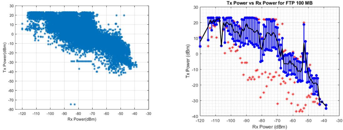
**Figure 54, UMTS TX vs RX power for CS, VoIP (skype), 10 MB file transfer and 100 MB file transfer. Blue dots on left figures represent measurement points. on the right figures, red dots represent the minimum and maximum measured values, blue lines the standard deviation and black line represent the mean.**
