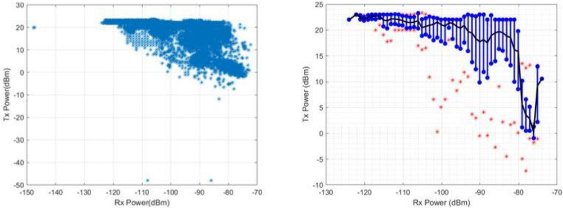
**Figure 24, UE TX vs RSRP for LTE technology in Basel campaign, on the left scatter plot and on the right red dots represent the minimum and maximum values, blue lines represent the standard deviation and black lines represent the average value**
