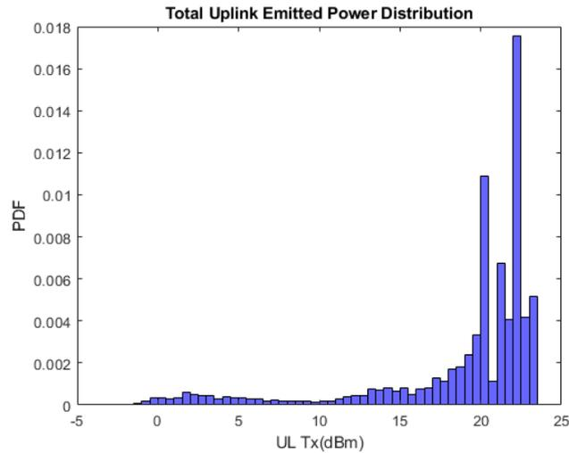
**Figure 25, PDF of measured UL emitted power for all measurements**
