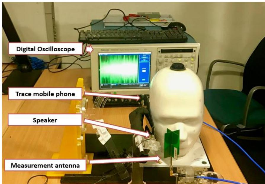
**Figure 51, Temporal UE TX power measurement configuration**
