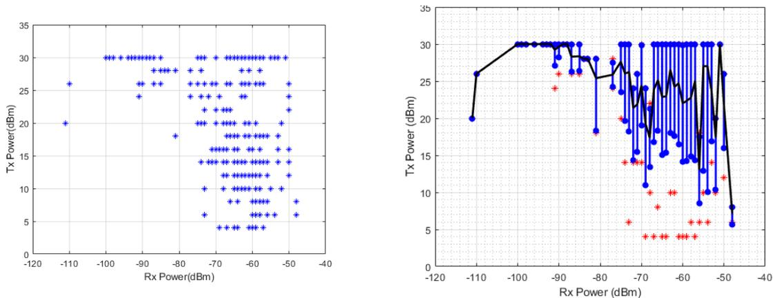
**Figure 55, GSM TX vs RX power for CS. Blue dots on the left figures represent measurement points. on the right figures, red dots represent the minimum and maximum measured values, blue lines the standard deviation, and black lines represent the mean value.**
