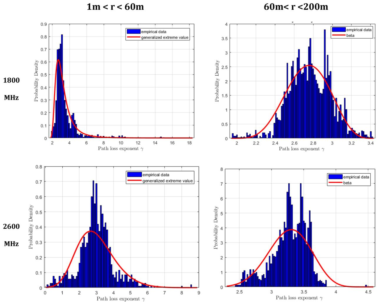
**Figure 43, PDF, distribution of measured PLE for 1800 and 2600MHz frequencies and for distances closer than 60m and further than 60m from the SC**
