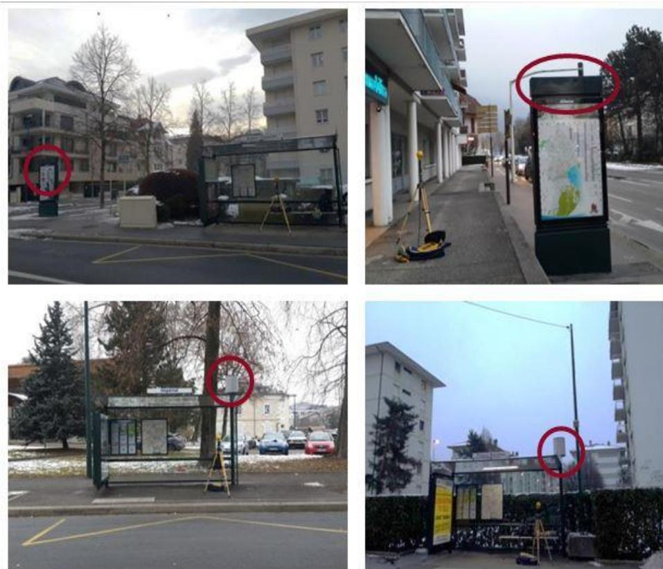
**Figure 27, SCs in Anancy under measurement and the location of measurement antennas at fixed positions for stationary measurements**
