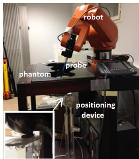
**Figure 13, SAR measurement setup**
