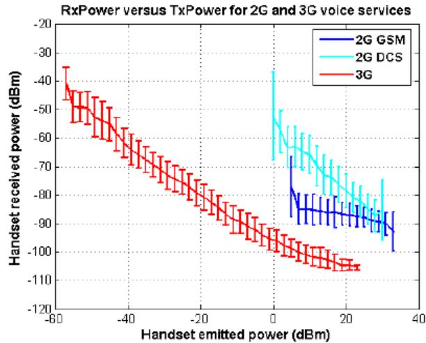
**Figure 17, the measured received power by UE in terms of uplink emitted power in GSM (blue curve), DCS (light blue) and UMTS (red), vertical lines represent the standard deviation and the horizontal line the average RX [4]**
