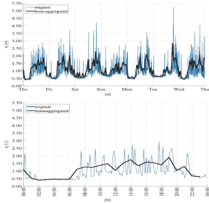
**Figure 15, Relative total electric-field strength measured during one week (a) and one day (b)[63]**
