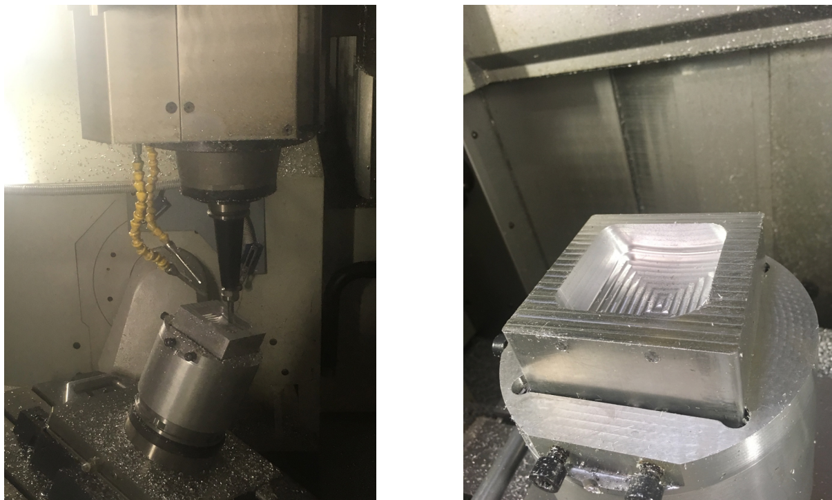
FIGURE 2.45 – Usinage de la poche test
