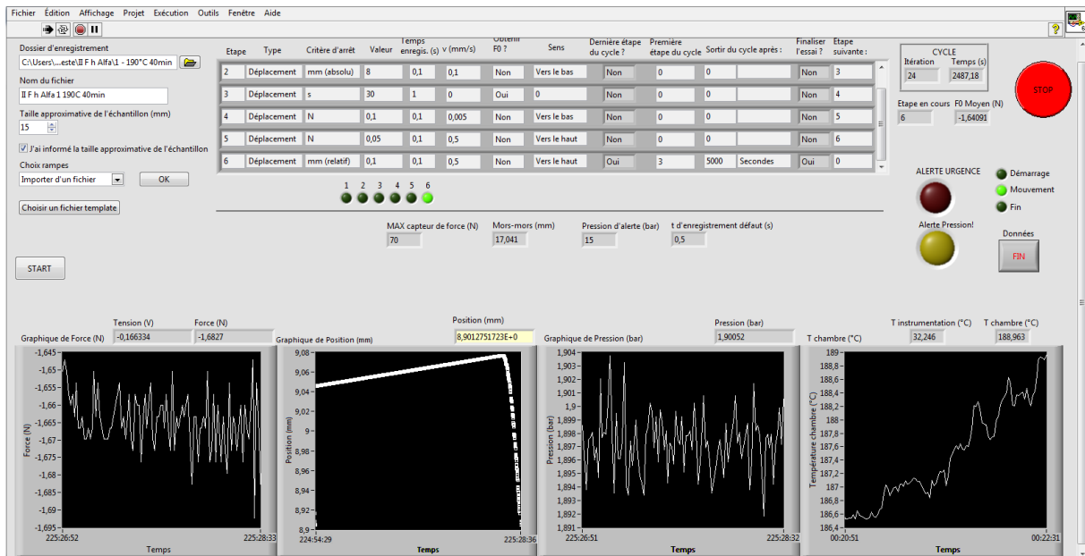
Figure 38. Overview of the control software (user interface).
