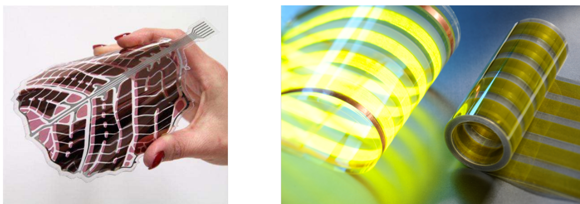
Figure 1: Examples of flexible devices: solar cells (left) and OLED (right) (Source: VTT, Technical Research Centre of Finland)
