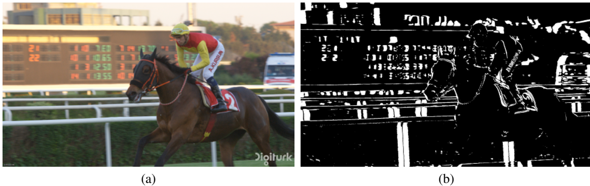
Fig. 7.5 Example of thresholded motion difference with (a) the original image of the Jokey sequence and (b) the thresholding activation map with threshold Th = 25 .
