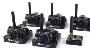
FIGURE 7.4: Picture of the Beacon indoor positioning system used for measuring array and loudspeaker 3D position.
