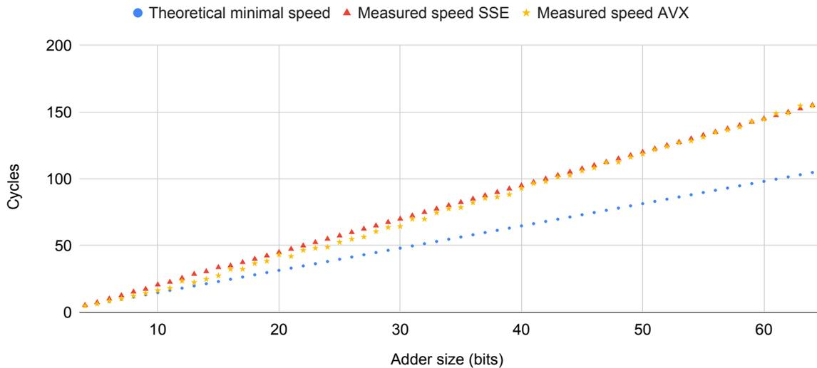
Figure 1.17: Scaling of bitsliced adders on SIMD
