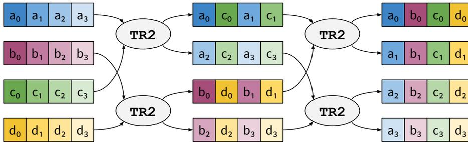
(b)  $4 \times 4$  matrix transposition using `tr2`
