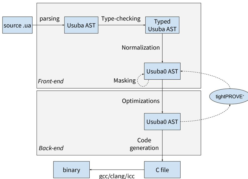
Figure 4.1: Usubac’s pipeline
