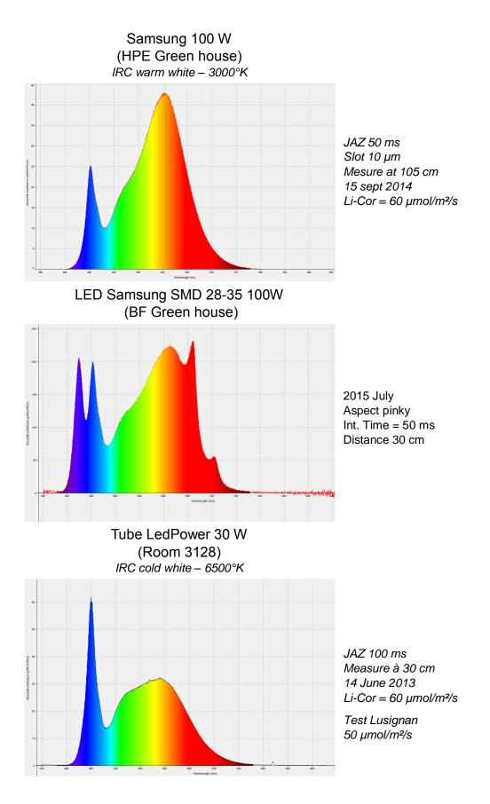
Figure 17: LED spectrum used in the greenhouses and the growth chamber.
