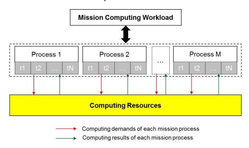
FIGURE 3.3: Mission computing workload. On the computing platform, a robotic mission is a multi-process workload. Each mission process is also a multi-thread workload. (Note: *t*1, ..., *tN* is thread)
