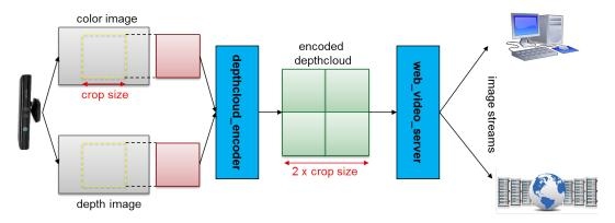
FIGURE 3.16: Video Server Mission. Its functional requirement is to provide the visual information of the working environment in the form of encoded depthclouds for the users.
