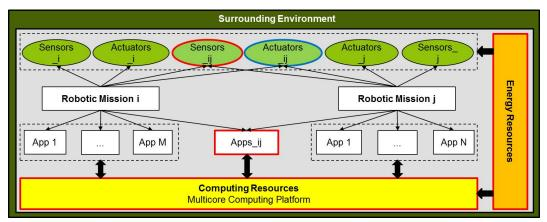
FIGURE 3.8: Multi-Mission context. Here, two example missions i and j can share resources (sensors, actuators, computing resources) and energy in a mutex locked (blue contour) or superposed manner (red contour).
