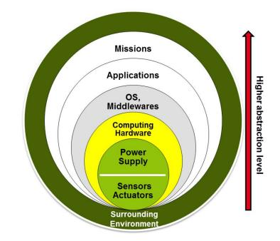
FIGURE 2.2: Abstraction level of mobile robotic systems in which the mission is at the highest level and the sensors and actuators are at the lowest one. All the system interacts directly with the surrounding physical environment.
