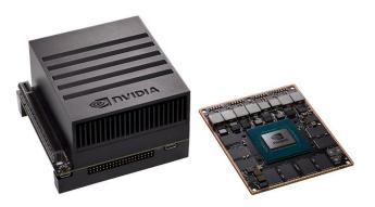
FIGURE A.1: NVIDIA Jetson AGX Xavier (reprinted from NVIDIA).
