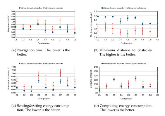
FIGURE 3.15: Characterization results of a navigation mission in terms of performance and energy consumption. The results are also compared between two different environmental contexts: without and with dynamic obstacles.
