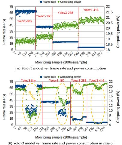
(B) Yolov3 model vs. frame rate and power consumption in case of person appearance
