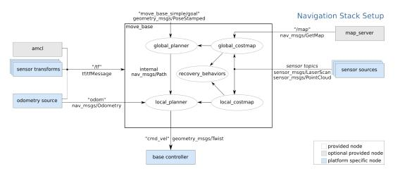
FIGURE 3.14: Autonomous Navigation Mission based on a ROS Navigation Stack. Its functional requirement is to visit a user-defined set of waypoints in the working environment based on a global map.
