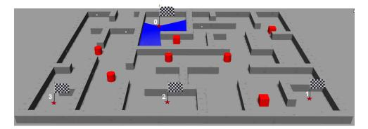
FIGURE 4.12: Example of a simulation environment in Gazebo with 7 dynamic obstacles: single box or cylinder in red models dynamic obstacles, blue area represents laser scan. The flags represent the examples of navigation waypoints.
