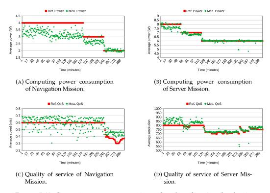
FIGURE 5.10: Computing power consumption and quality of service of each mission controlled by the Multi-Mission Manager. The red points indicate the reference values or the adaptation request (computing power budget, desired quality of service) of each mission. The green points are respectively the measured values (averaged during an episode of 1 minute of each Mission Manager) of each mission.
