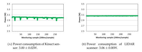
FIGURE D.2: Estimated power consumption of Kinect and LIDAR sensors using Yocto-Watt.
