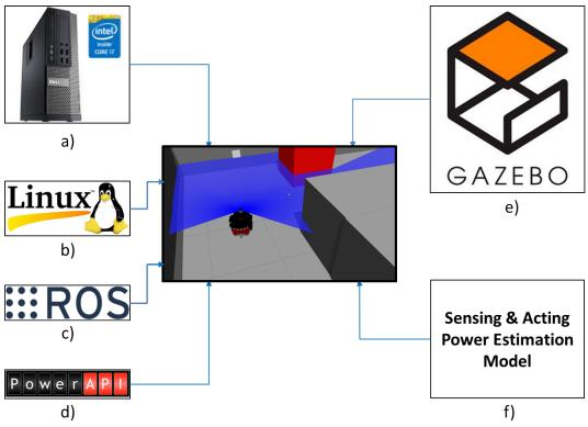
FIGURE 3.12: Simulation framework: a) Intel Core i7 desktop, b) Linux-based operating system, c) Robot Operating System, d) PowerAPI, e) Gazebo simulator and f) Sensing & acting power estimation model.
