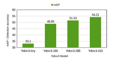
FIGURE 3.20: Detection accuracy of four Yolov3 models.
