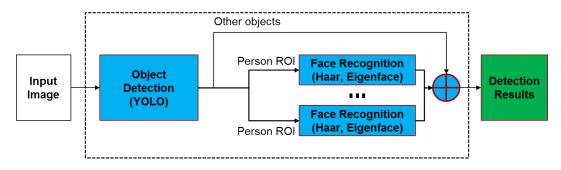
FIGURE 3.18: Semantic Environment Understanding Mission. Its functional requirement is to understand the scene by detecting and recognizing the objects and people in the robot's working environment.
