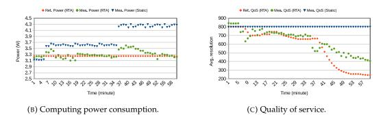
FIGURE 6.9: A comparison between run-time adaptation and static configuration of the video server mission. From 1 to 5 minutes: 1 visualization request of  $512 \times 512$ . From 6 to 35 minutes: 2 visualization requests of  $512 \times 512$ . From 36 to 60 minutes: 2 visualization requests, one of  $512 \times 512$  and another of  $1024 \times 1024$ .
