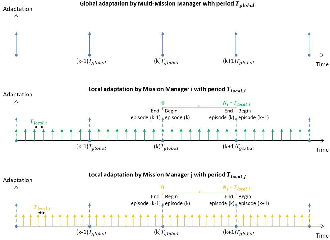
FIGURE 5.5: Timing synchronization between Multi-Mission Manager and Mission Managers. Each Mission Manager has its local adaptation period. The episode of each Mission Manager is then synchronized with the global adaptation period of the Multi-Mission Manager.
