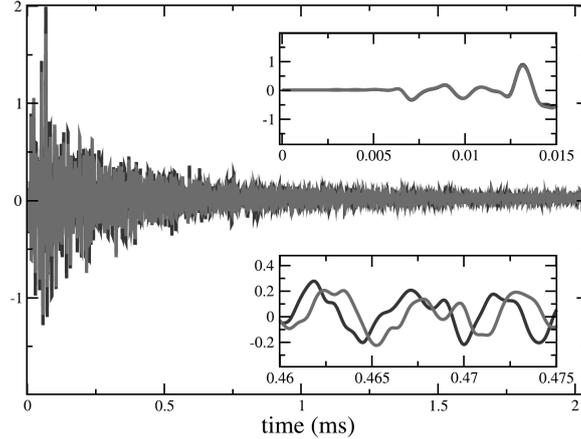
Figure 3.1: Recorded waveforms in a sample of granite for two different temperatures, 45°C (gray) and 50°C (black). The top inset shows the waveforms at these two temperatures around the direct arrivals and the bottom one shows the one for the part of coda arrivals (Figure from [66]).
