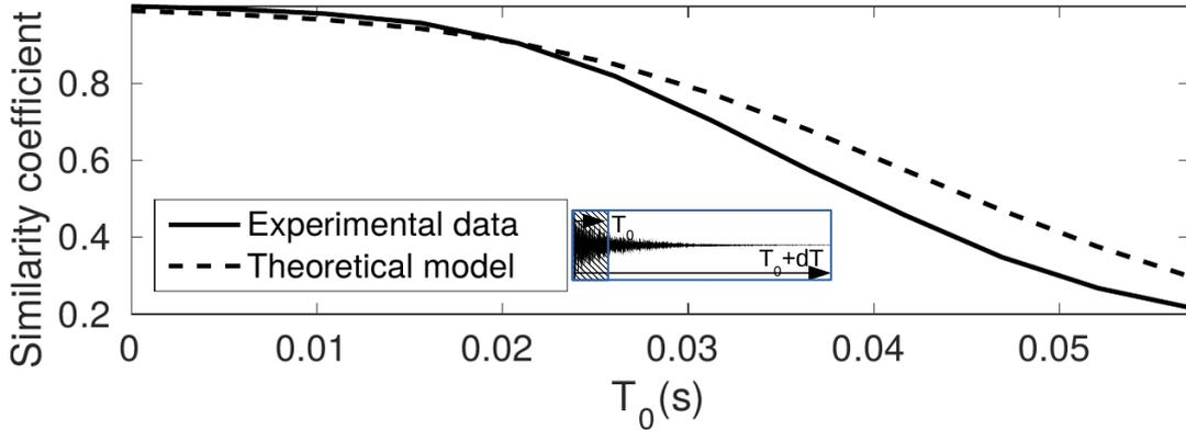
Figure 2.18:  $S(C_\infty, C_\infty^{dT})$  between  $C_\infty(\mathbf{r}_l^R, \mathbf{r}_{l'}^R, t)$  and  $C_\infty^{dT}(\mathbf{r}_l^R, \mathbf{r}_{l'}^R, t)$ . The end of the time windows ( $T_0 + dT$ ) is fixed at 250 ms.  $S(C_\infty, C_\infty^{dT})$  is then evaluated in a window that includes direct path and primary coda ( $\Delta\theta = 2$  ms).
