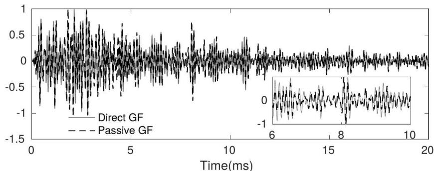
Figure 3.7: Comparison between actively (gray solid line) and passively (black dashed line) retrieved Green's functions bandpass filtered from 5 kHz to 10 kHz and normalized by maximum amplitude. The inset shows the zoom from 6 ms to 10 ms that corresponds to  $\sim 4$  m of propagation in the reverberating plate.
