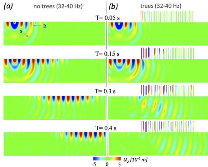
Figure 4.13: Results of the numerical simulations for the  $u_z$  component of the recordings at different times, and for two different set-ups: (a) half space without trees; (b) half space with trees. The recordings are filtered in the first bandgap. R and S indicate Rayleigh and S waves (Figure from [103]).
