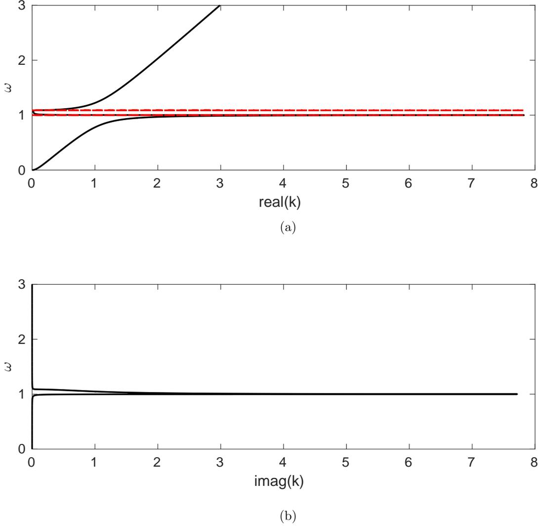
Figure 4.4: Frequency-wavenumber representation of the real (a) and imaginary (b) parts of the wavenumber for a system consisting of a set of resonators. The resonance frequency of each single element is 1 rad/s and the wave propagation speed is 1 m/s. Horizontal red lines mark the frequencies of start and end of the bandgap.
