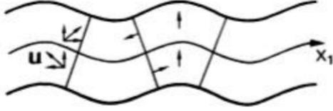
Figure 1.3: Fundamental antisymmetric Lamb wave (Figure from [3]).
