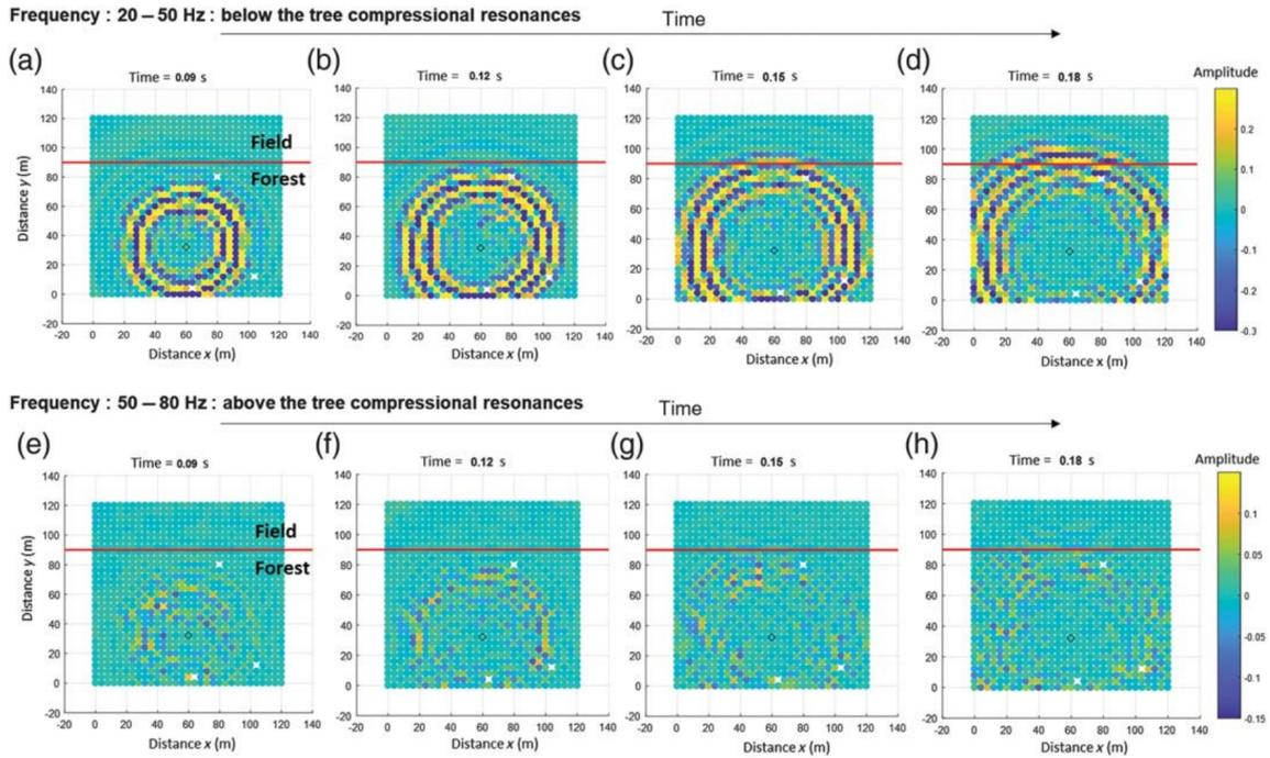
Figure 4.18: Measured seismic wave-field inside the forest on a 2D array of one-component Z-land receivers, with the excitation source at  $x = 60$  m and  $y = 30$  m (i.e., inside the forest). The temporal evolution of the wave-field filtered between 20 Hz and 50 Hz (a-d) and between 50 Hz and 80 Hz (e-h) are shown. The horizontal red line indicates the field-forest boundary (Figure from [104]).
