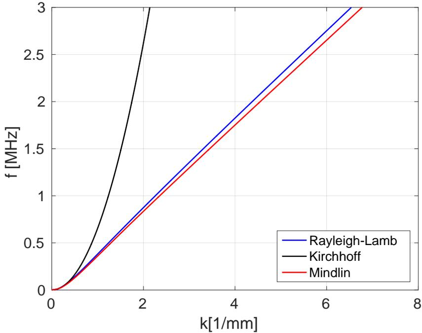
Figure 1.7: Frequency-wavenumber representation for  $A_0$  mode obtained from three different approaches: exact theory of Rayleigh-Lamb (blue curve), theory of Kirchhoff (black curve) and theory of Mindlin (red curve) for a duralumin plate of thickness of 3 mm.
