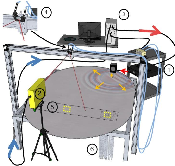
Figure 4.5: Experimental set-up in the study of  $[100]$ , consisting of: (1) a shaker to excite the  $A_0$  mode of the Lamb waves in the aluminum plate; (2) a laser Doppler velocimeter to measure the wave-field on the plate; (3) a computer to control the set-up; and (4) a motorized mirror. The scan of the surface of the plate is performed over rectangle 5, and the metamaterial region is constructed by attaching the vertical aluminum rods, marked as 6 (Figure from [100]).
