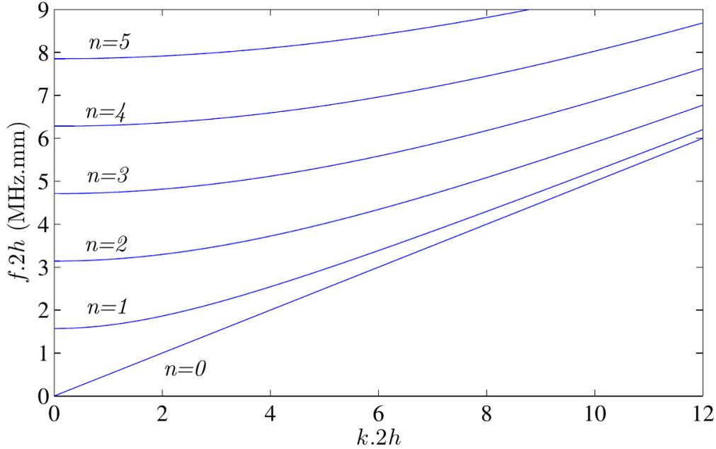
Figure 1.5: Frequency-wavenumber representation for  $SH$  waves based on Eq. 1.2. The plate is infinite and made of aluminum. Poisson coefficient and speed of transverse waves are 0.34 and 3140 m/s, respectively (Figure from [4]).
