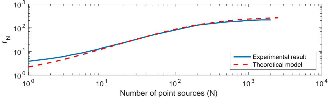
Figure 2.13:  $r_N$  as a function of the number of sources  $N$  picked randomly, derived from the experimental data (blue line) using Eq. (2.32), and modeled (dashed red line) based on the theory developed and summarized by Eq. (2.40). A 4th order Butterworth filter between 5000 Hz and 15000 Hz is applied to experimental data.
