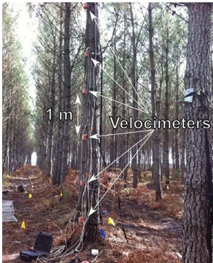
Figure 4.19: A tree with six three-component velocimeters attached to its trunk at different heights (Figure from [104]).
