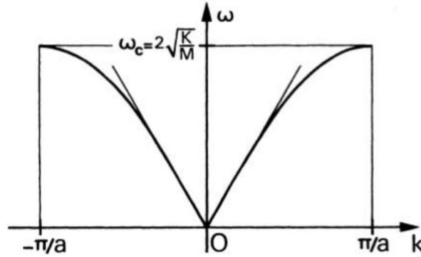
Figure 4.2: Dispersion curve for the waves that propagate in a one-dimensional array of atoms (as shown in Fig. 4.1).  $\omega_c$  is the cut-off frequency, below which two modes can propagate in opposite directions (Figure from [3]).
