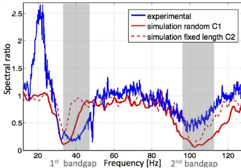
Figure 4.11: Experimentally measured (blue curve) and numerically simulated (red curves) spectral ratios. Solid and dashed red lines correspond to the configurations  $C_1$  and  $C_2$  (Figure from [103]).
