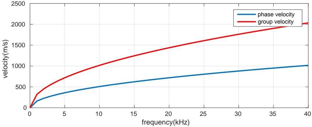
Figure 1.6: Dispersion curve for  $A_0$  Lamb mode as a function of frequency. The thickness of the plate is 3 mm. The curves are obtained according to Eq. 1.7 for phase (blue curve) and group (red curve) velocity.
