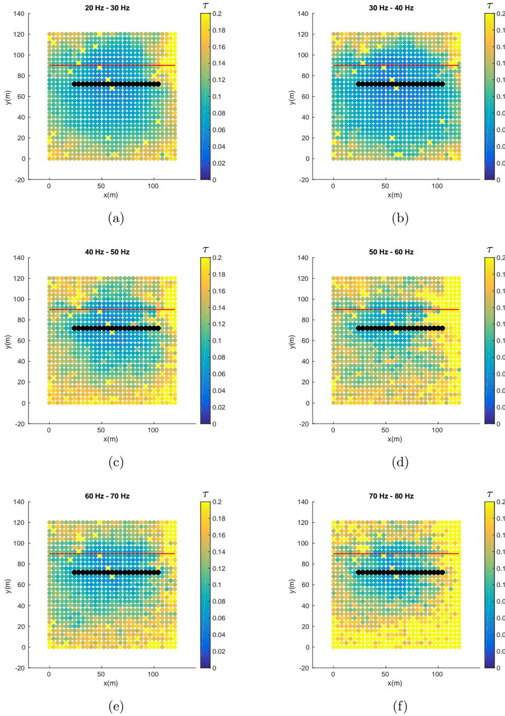
Figure 4.34: Spatial map of the spreading time of the signals ( $\tau$ ; in seconds) computed according to Eq. 4.23 along a horizontal line of virtual receivers inside the forest and from virtual sources that are arranged with regular spacing in the field and the forest and in different frequency bands.  $\tau$  is averaged over all of the possible virtual receivers. Black circles mark the positions of the virtual receivers.
