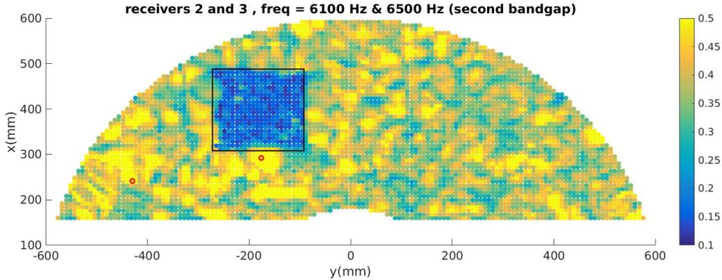
Figure 4.24: Spatial distribution of the maximum of the normalized cross-correlation of recordings at two virtual receivers (marked by red circles) from each virtual point source for data filtered within the second bandgap (between 6100 Hz and 6500 Hz) prior to cross-correlation. The black square marks the metamaterial region. Both of the virtual receivers are located outside the metamaterial.
