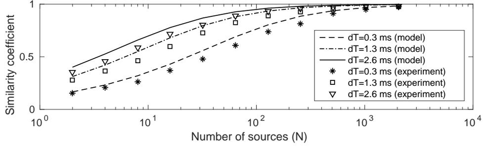
Figure 2.16: Similarity coefficient  $S(C_\infty, C_N^{dT})$  between  $C_\infty$  and  $C_N^{dT}$  (cross-correlation obtained by windowing one signal before the cross-correlation, and then averaged over a subset of available sources picked at random). Symbols and lines show the experimental results and theoretical model, respectively, for the various window lengths ( $dT$ ). The starting time ( $T_0$ ) in all three cases is 2.3 ms, i.e., no ballistic signal is cross-correlated.
