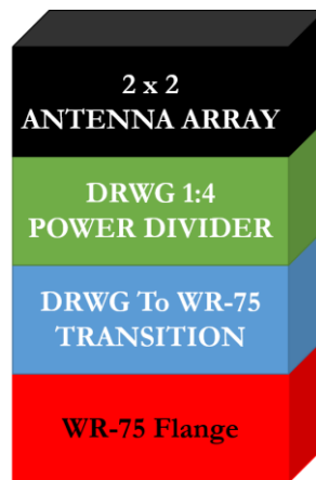
Figure 87 Integration scheme for the 2x2 DRWG sub-array with corporate feeding network and WR-75 flange.
