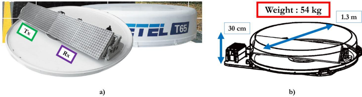
Figure 7 Sanetel T65 SOTM user's terminal integrating slotted waveguide array antennas working at Ku-band: a) picture of the terminal from [25], b) schematic of the T65 antenna solution with radome from [25].
