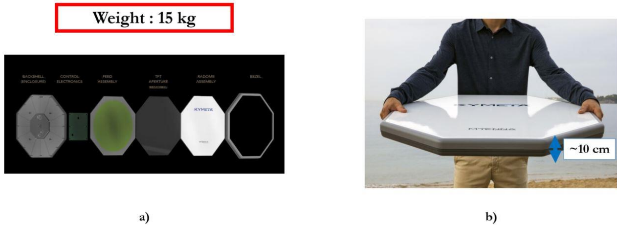
Figure 10 a) Exploded stack-up of the Kymeta antenna panel from [30], b) picture of a Kymeta panel from [29].
