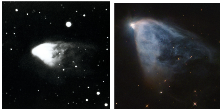
FIGURE 2: Images of NGC 2261 taken with the Hale telescope in 1949, and by the Hubble Space Telescope in 1999. Even though the Hale telescope is twice the size of Hubble, it produces less sharp images. The atmosphere explains this difference: the 1949 image is limited by atmospheric effects, while the 1999 Hubble image is diffraction limited.
